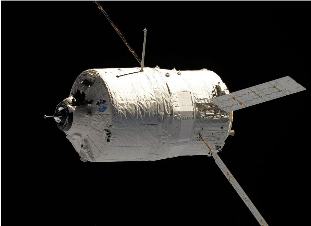
Automated Transfer Vehicle - ATV1 (4.5 m diameter, 9 m long)
