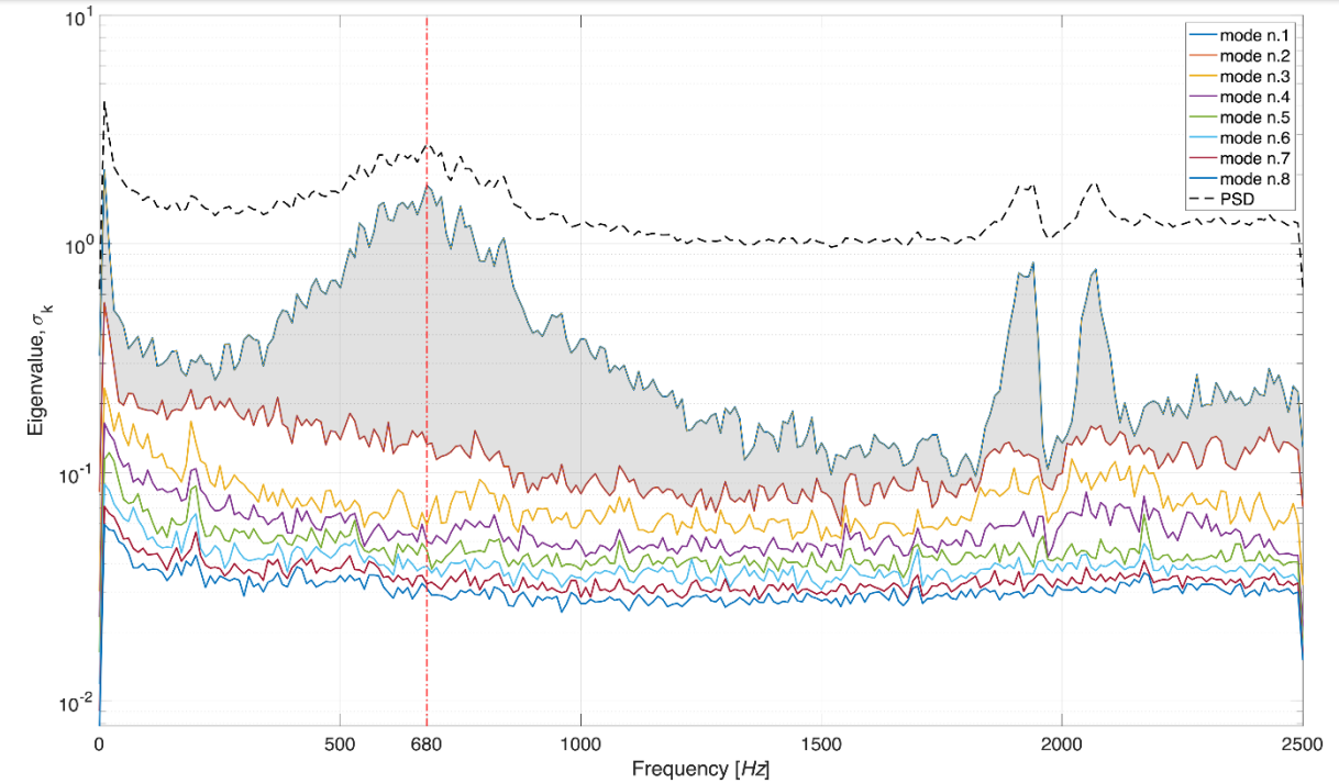
SPOD energy spectrum for subcritical mode , sidewall-test case
