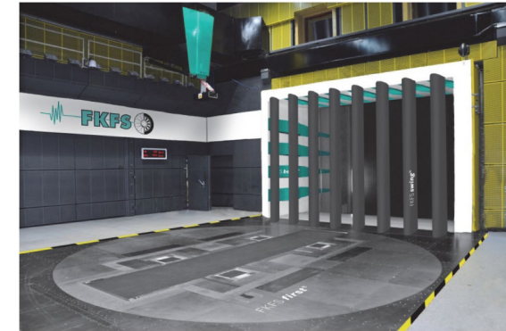
MOVING GROUND AND TURNTABLE; TRAVERSE; TURBULENCE GENERATION [1]
