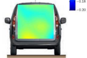
Fig. 22. Conditionally averaged base pressure distribution C_p(y^*, z^*) for the Renault Kangoo ( \beta = 4.0^\circ ): (a) State T - (b) State B
